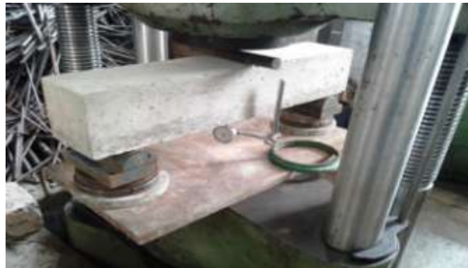
Figure 5. Test setup for one point loading test.
