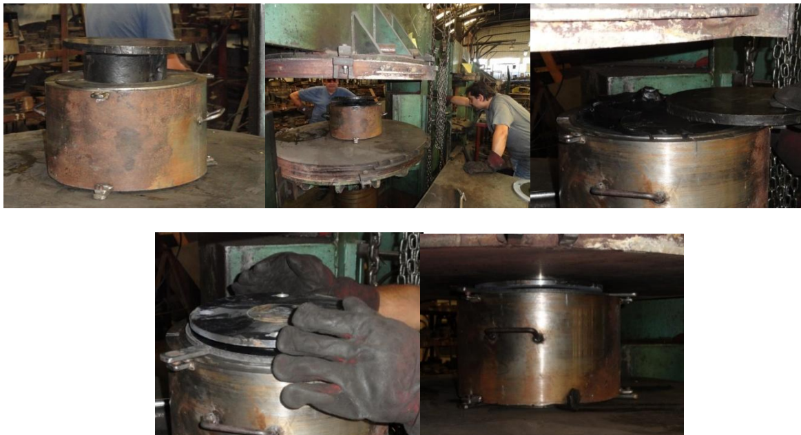
Figure 12. Devices prior to vulcanizing process. Vulcanizing process and positioning of the upper connection plate and final vulcanization.
