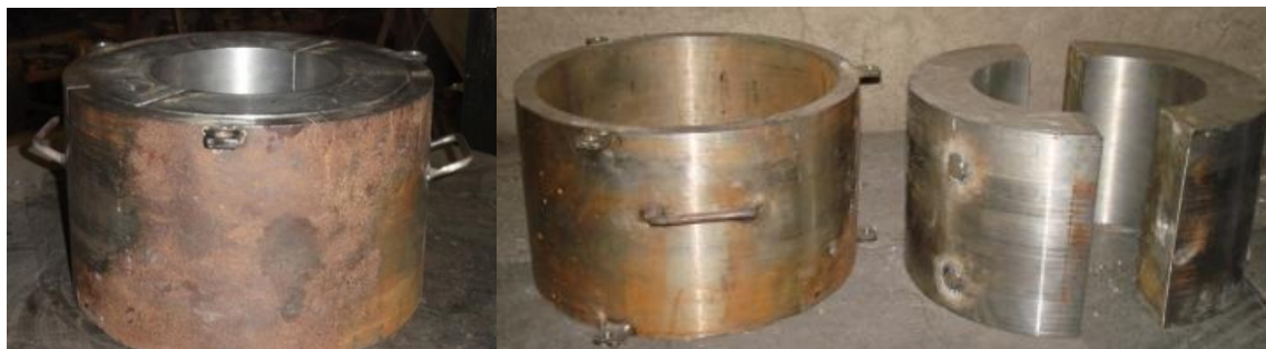
Figure 7. Molds used in the manufacturing of the seismic isolation devices
