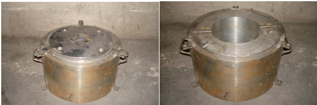
Figure 10. Molds, connection plates and centering ring.
