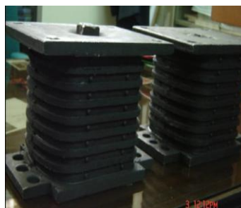
Figure 3. Devices manufactured in Ecuador with elastomers of disused tires.
