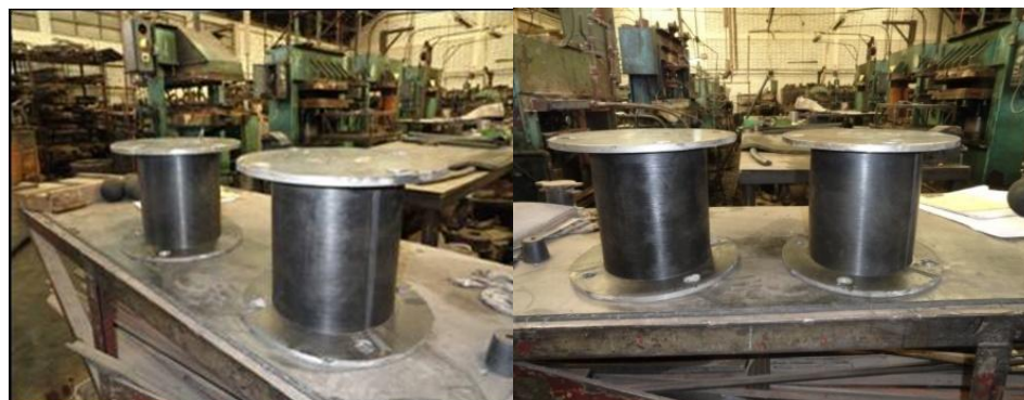
Figure 13. Removing the seismic isolation devices.
