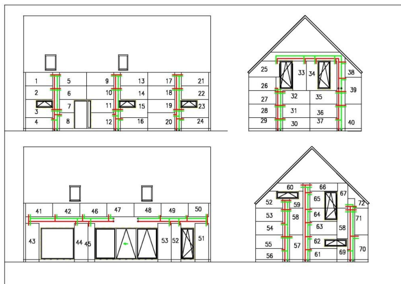
FIG. 4 Principle of construction of a contact thermal insulation system using thermal insulation panels with ATP (WATER as the heat-transfer medium) (author: Kalús)
