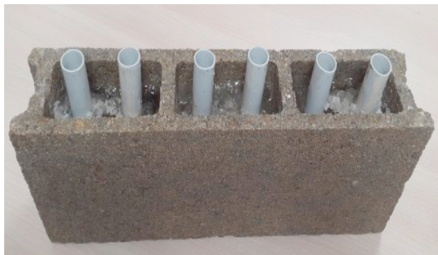
Figure13: Concrete block with PCM and ventilation tubes [54].
