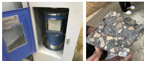
Figure 4: Compressive strength testing of concrete cubes
