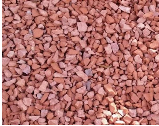
Figure 3: Low – quality crushed brick aggregate
