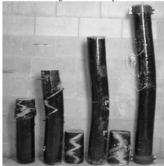
Figure 3. Different failure modes of the slender CFST columns.
