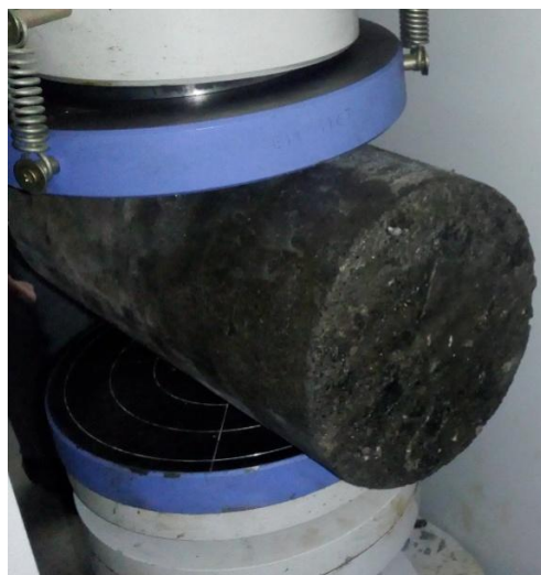
Figure 5 Determination of Split tensile Strength of concrete
