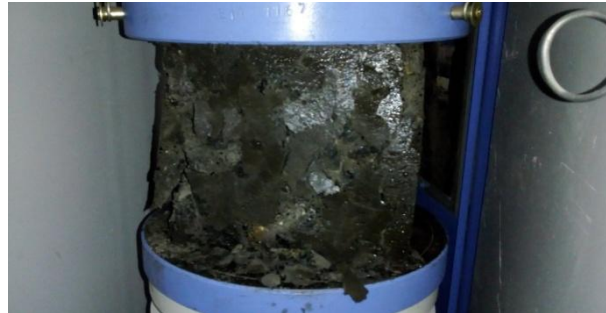
Figure 4 Determination of Compressive Strength of concrete
