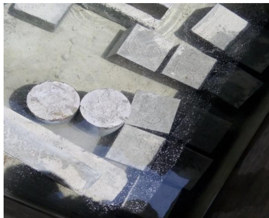
Figure 3 Curing of concrete cubes,
