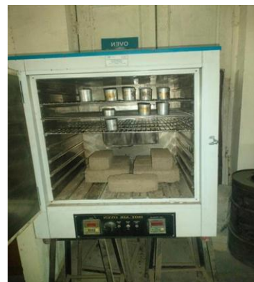
Fig. 3.4. Bricks for firing in the kiln
