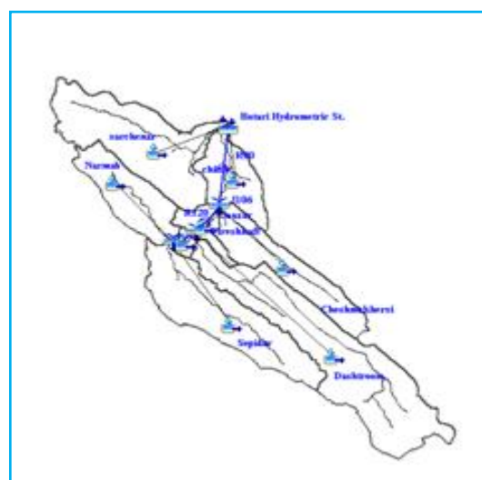
Fig 3. Processed results for Semi- Distributed Basin imported to HEC- HMS for simulation
