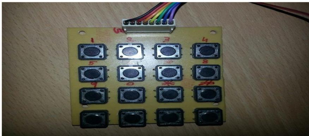
FIG 4: ATMEL MICROCONTROLLER-BASED KEYBOARD
