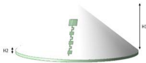
Figure 6: Patch Antenna embedded In Cone
