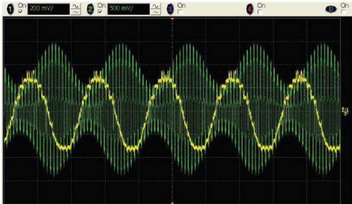
Figure 12: Input and Output waveforms of the AM demodulator
