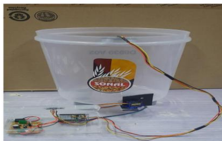
Fig. 3: hardware setup of Animal feeder
