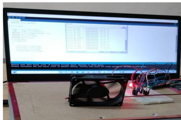
Fig.5: Fan turns ON and Indication is given through RED LED when the detected temperature is greater than the set temperature
