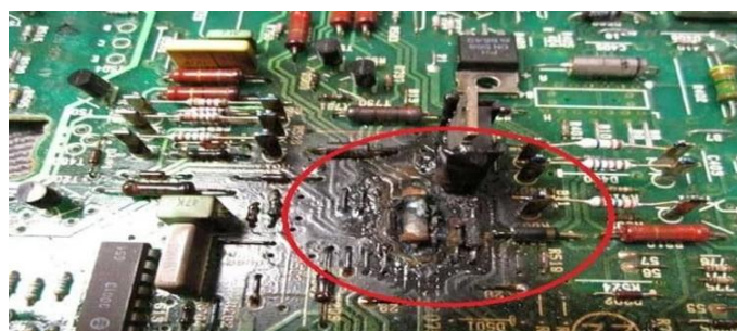
Fig.1: Damaged Internal Structure of the Electronic Device due to Overheating
