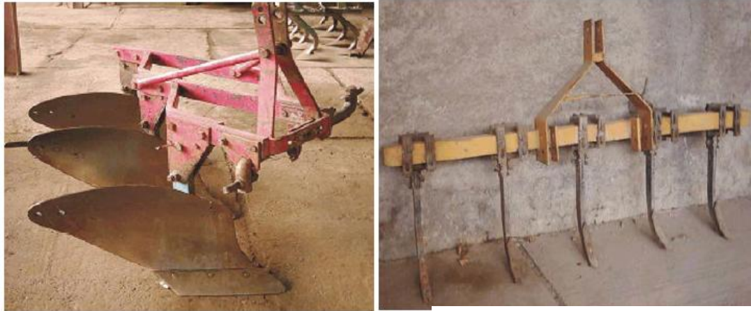
Plate 6: Moldboard Plow: The moldboard plow was a three furrow mounted plow. Furrow width was set to 365 mm and plowing depth was set to 250 mm.
