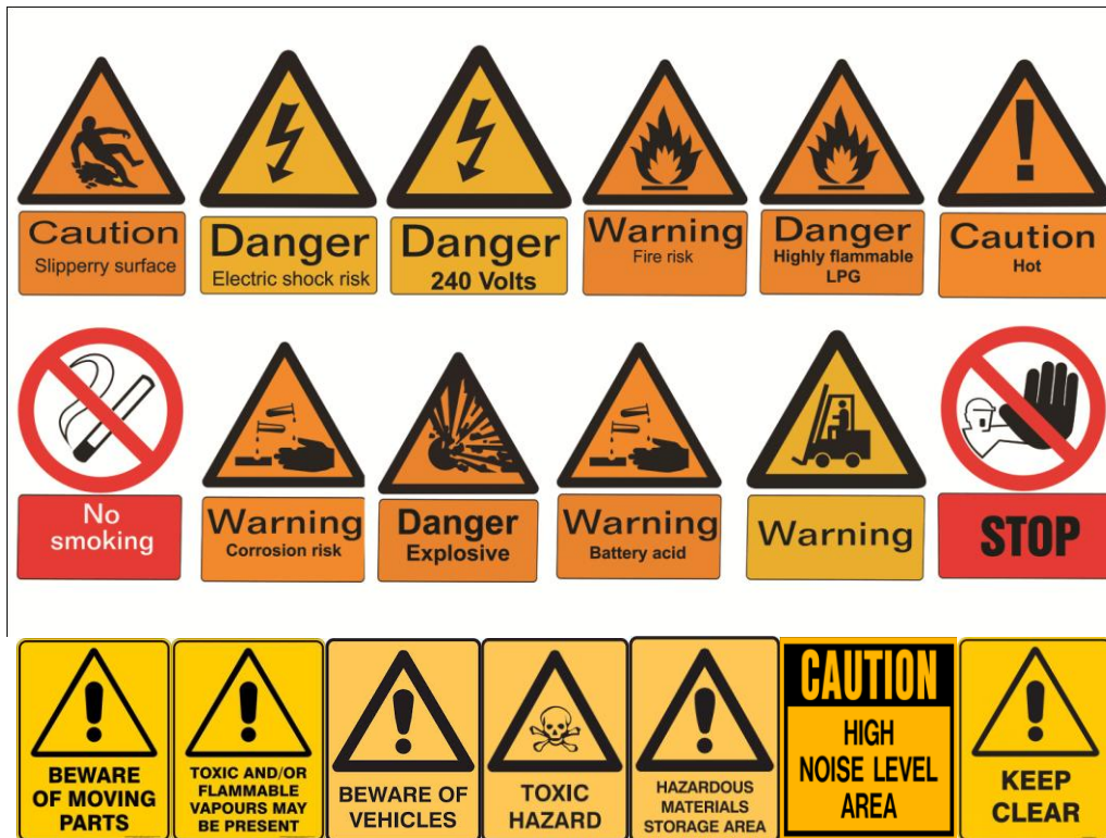
Figure 1. Danger, warning and caution safety signs[20]
