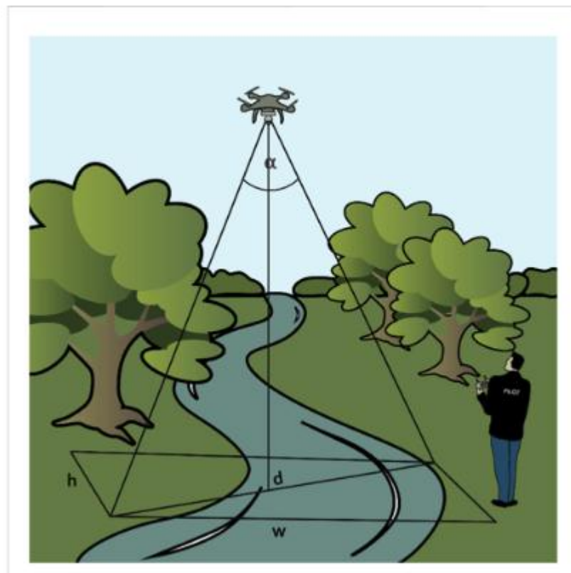
Figure 1: Visualization of the use of the drone when taking recordings by the camera that is positioned towards the ground. The drawing also overlays the data used to perform georeferencing, such as: width w and height h of the image, the height of the drone H and the field of view as the \alpha angle.
