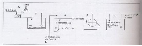
A filtering system (A) which filters large solid particles in suspension
