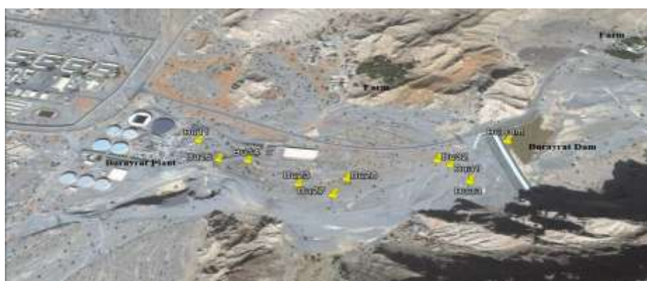
Photo 4. Al Burayrat desalination plant and surrounding human activities may represent potential sources of groundwater pollution in the study area. Percolation of surface water from Al Burayrat dam reservoir can contribute to bacterial pollution of Wadi Al Bih limestone aquifer.
