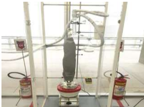
Figure 3 – Packed Distillation Column.
