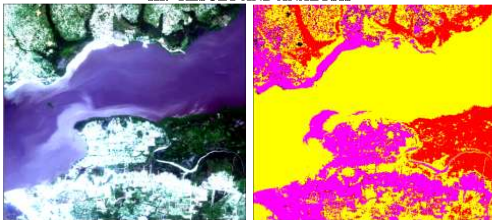
Figure 10: Side-by-side comparison/identification of spectral signature with Magenta as soil, Red as vegetation and Yellow as deep-shallow water.
