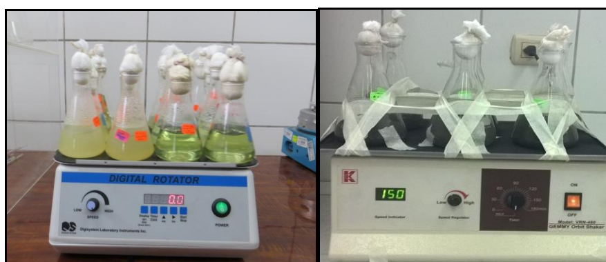
Figure 3.4.1. Beginning of the first stage of bioleaching, at different \text{FeSO}_4 \cdot 7\text{H}_2\text{O} concentrations.
