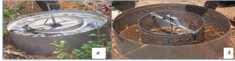
Figure 2: Double ring infiltrometer experiment at the beginning and end of experiment
