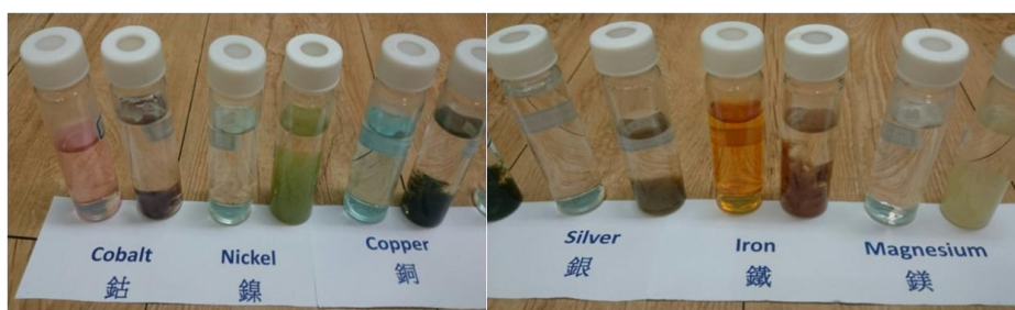
Fig. 1. Color change of LCW fiber after adsorption of heavy metals
