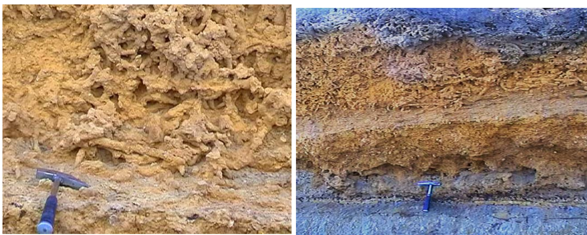
Figure-14 Field Photographs of Vinjianian Carbonate in Kutch On land (Analogues of L-III carbonates of Mumbai High) showing Interstratified Layers of: Highly Bioturbated Carbonates- Non-bioturbated wackestone/packstones Argillaceous/Micritic Limestone Shale/Clay horizons. Right panel shows the zoomed image of intergranular porosity created by bioturbation.
