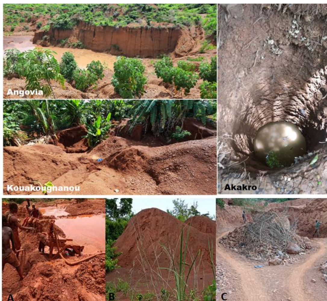
Figure 3: Physical impact of gold mining activities on the ground showing gold extraction pits from deep eluviums and unrehabilitated sites. A: treatment sludge; B: waste rock dump; C: surface excavation quarry.
