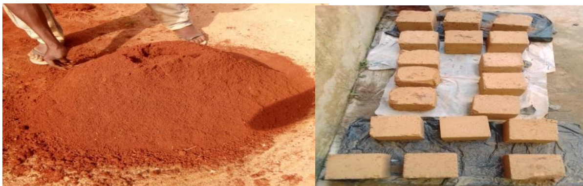
Fig 1. Pictorial view of soil sample & manually compressed earth bricks. Source: Joseph & Olugbenga, (2020).
