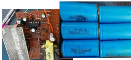
Figure 2.2: On Board Complete Circuit and Arrayed Lithium Battery
