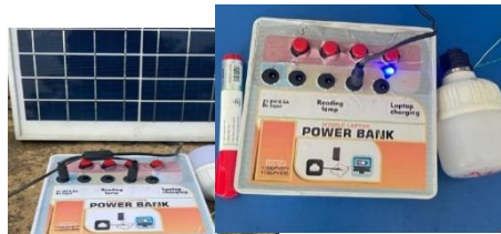
Figure 2.3: Complete Solar Power Laptop Bank
