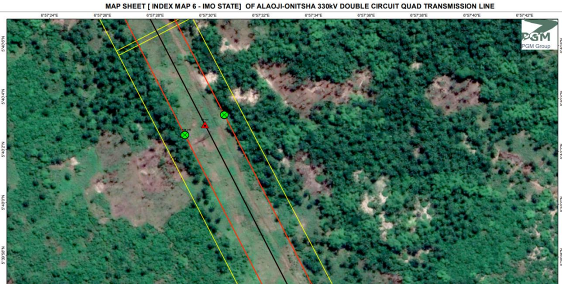
Figure 7: Constraint map showing zero ROW encroachment at 50 m at Agbala (same throughout NgorOkpalla LGA in Imo and Osisioma LGA in Abia State (Source: RAP Report of the Alaoji-Onitsha TL, 2019)
