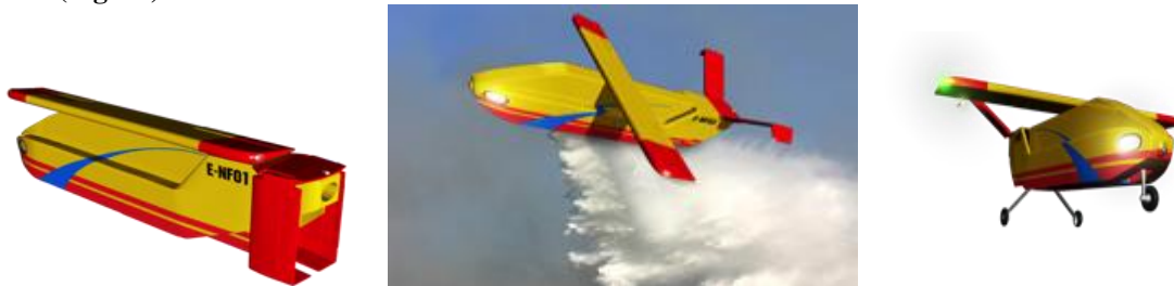
Fig. 15: NitroFirex AGC, s configurations (on board, flying /dropping, landing / on ground)
