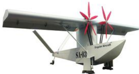
Fig. n° 13: unmanned propeller bi-motor hydroplane
