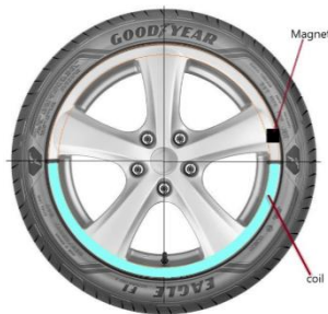
Figure 2. simple drawing about placement of magnetic and coil
