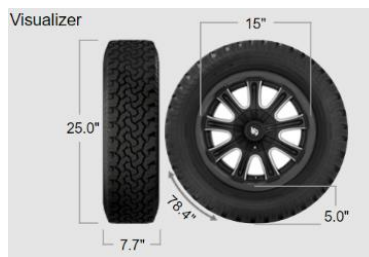
Figure 1. characteristic of Goodyear wheel 196/65R15''
