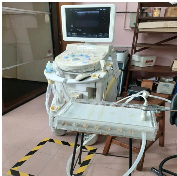
Figure 2: Ultrasound measurements of hemodynamic parameters using the Hitachi ultrasound machine
