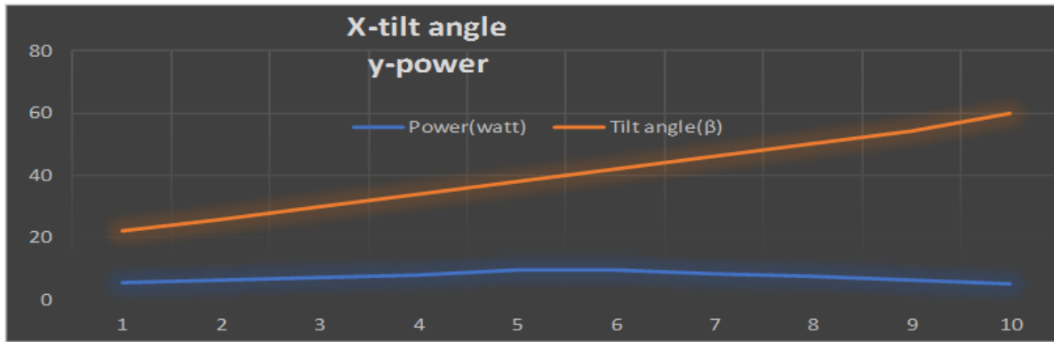
Figure 4: increase the angle gradually, power is first increases then decreases.
