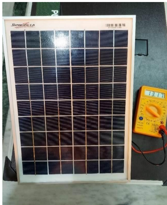
Figure 1: Setup of PV module calculating current and voltage
