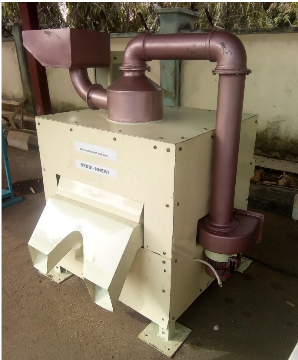
Plate 3: Double Screen novel Rice Destoning Machine
