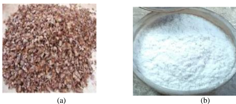
Figure 1: The picture of (a) breadfruit seed coat (BSC), and (b) recycled low density polyethylene
